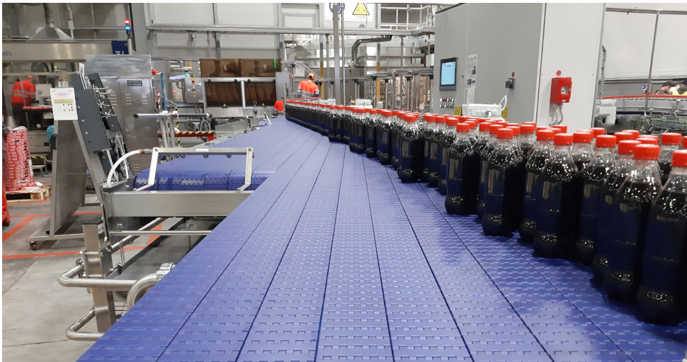
Figure 2.5. The enhanced tribology of Delrin® modified grades results in low wear, low friction and low noise
