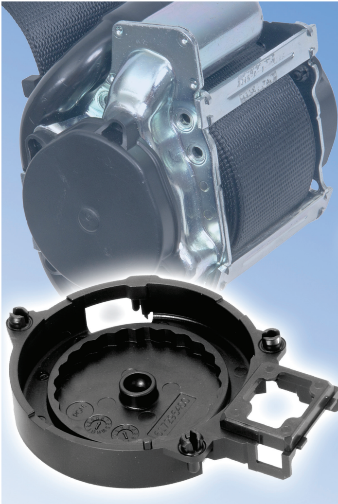
Figure 2.2. Autoliv safety belt retractor bearing plate made with Delrin® 300TE
